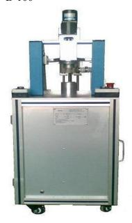
Model TP-B-100 is a semi automatic cosmetic pressed powder surface (convex surface) cleaning machine designed for the production of eye shadow, baked powder
