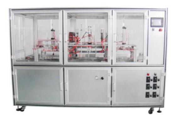
$Model\ TS\text{-}10A\ is\ an\ automatic\ lipstick/pencil\ releasing\ machine\ designed\ for\ the\ production\ of\ soft\ rubber\ lipsticks, lip\ balm.$
