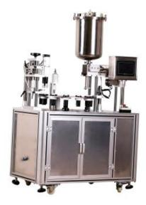
Model **TM-12-1** is an semi-automatic filling and capping machine design for the production of lip gloss and mascara
