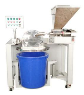
Model TP-P7.5Pis an automatic cosmetic powder disintegrator (pulverizer) designed for the crushing of raw material of eye shadow, blush, two way cake, and baking powder.
