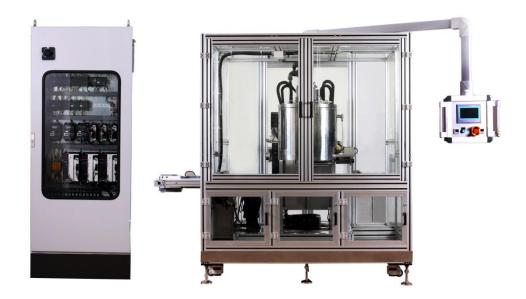
Model TL-50L-2-2A is an automatic double-nozzle hot filling machine designed for quantitative filling for lipsticks and other cream products in circle or square components.
