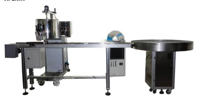
**Model TL-25L01** is a automatic filling machine designed for the production of godet and bottles filling product, lipstick, lip balm, eyeliner, liquid powder, and other hot pour products.
