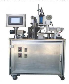
Model TP-B-01 is an automatic cosmetic baked powder pressing machine designed for the production of baked powder, such as eye shadow, blush and so on.
