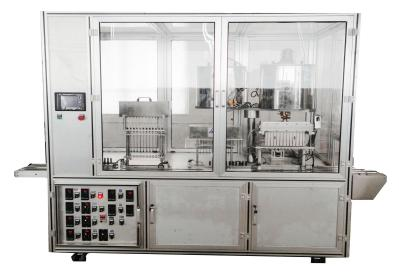
$\label{eq:model_TPF-10A} \textbf{Model TPF-10A} \ is \ a \ fully \ automatic \ aluminum \ molding \ machine \ designed \ for \ the \ production \ of \ cosmetic \ pencil \ .$
